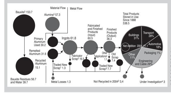
Figure 3. A material flow model for the global aluminum industry throughout its life cycle, developed by IAI for the year 2004. For additional details, see Reference 3, p. 95. Values cited are in millions of metric tons.
